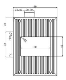
The NS5 is designed to be mounted on a DIN rail system. If your vessel does not have a suitable DIN rail system, use the supplied 100mm length of DIN rail. Secure the DIN rail to a flat surface in the selected location. Use two M4 wood screws or other fixings suited to the material the unit is being fixed to. The unit may be installed in any orientation
